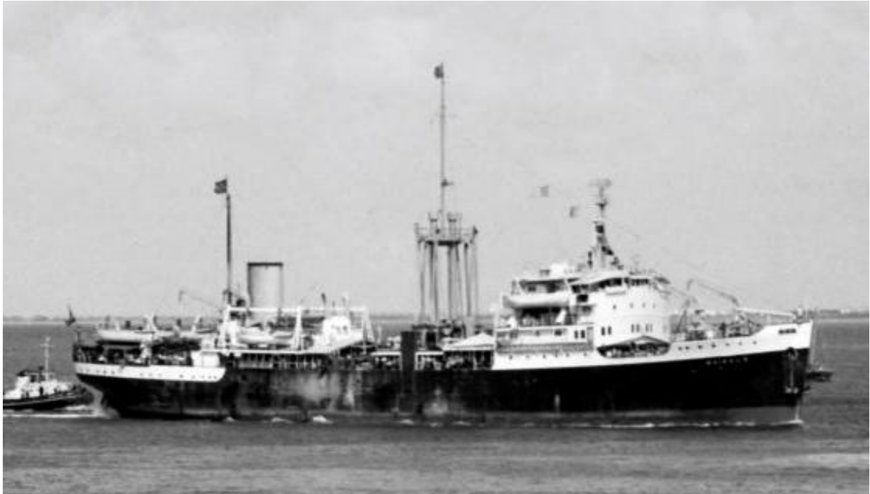
KPM's Waikelo arriving at Aden, 26 February 1962, with a large complement of deck passengers. First-class cabins forward, second-class aft (white section). Derricks topped at the mast (Dr. George Wilson).
