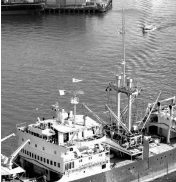
Midship section of Waingapoe in 1970 showing goalpost mast, large ventilators, and cattle ramp (raised) for access to the tweendeck with a row of portholes to give light for cattle or passengers. The big windows below the bridge could be fixed at horizontal for airflow to the first-class lounge and accommodation, being three 2-berth cabins on each side. The forward gooseneck cranes were a characteristic feature of the KPM's later 1930s-1950s vessels, as also the slewing, open-section jib cranes at the mainmast (John Mathieson/NAA).
