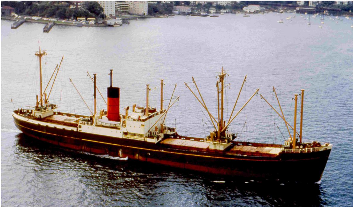
AN FU as KOMATA seen from Harbour Bridge departing from Sydney, 17 March 1966, in Union S.S. Co. colours and showing long hatches with retractable McGregor covers, being an early example (J.Y. Freeman/NAA).
