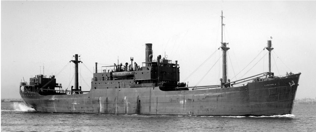
HANNAH MOLLER/MOUNT PARKER at Melbourne as ASB collier CARCOOLA with extra accommodation amidships and aft (A.G. Green/SLV).
